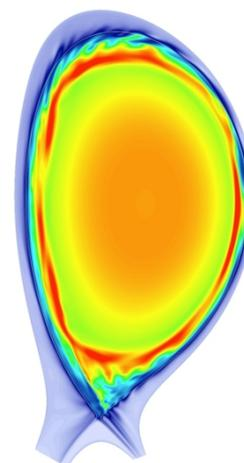
*Density profile in JET pellet triggered ELM simulation*
